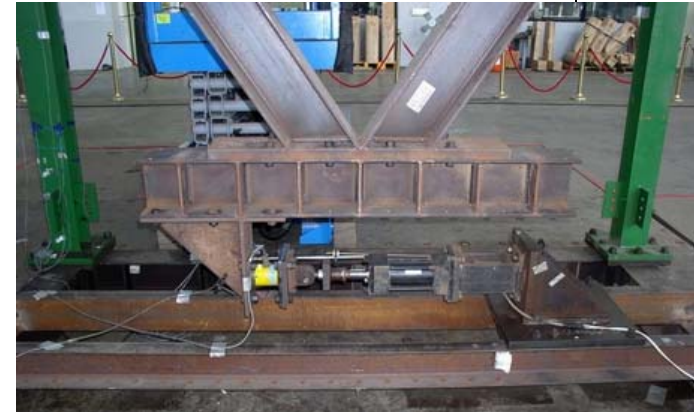
20 kN Magneto-Rheological (MR) Damper
